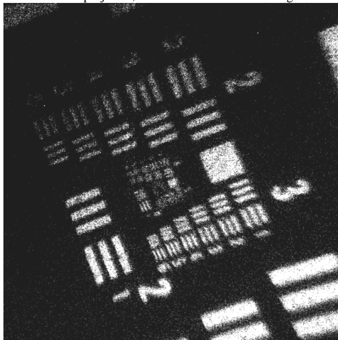
Figure 10. Projection of a standard USAF test target projected onto the detector.
